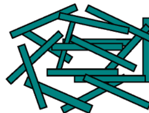
Figure 1. Schematic of the house-of-cards structure.
